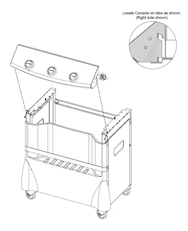
Note: Check wires from switch harness to ensure that they are not against any sharp surfaces.
